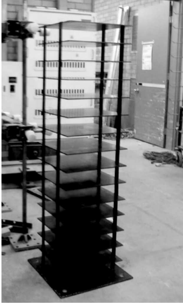
Figure 3.1. Shake Table Specimen Used by Tabatabaiefar et al.[69]
